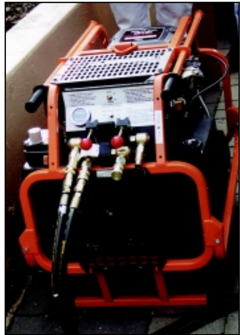
The portable hydraulic pump for driving the tools.
